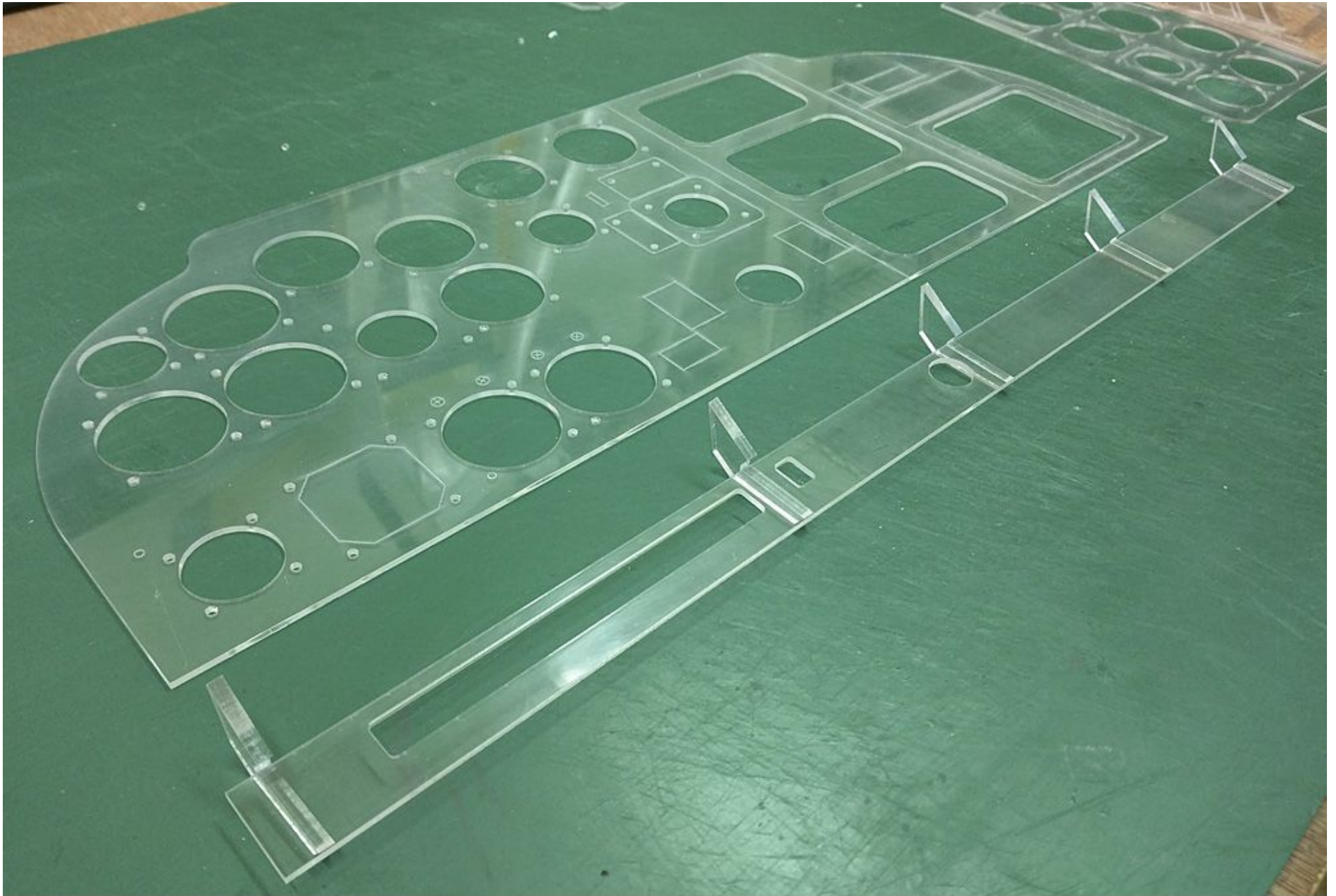
Angled brackets used to mount the subpanel to the main panel at an angle.
